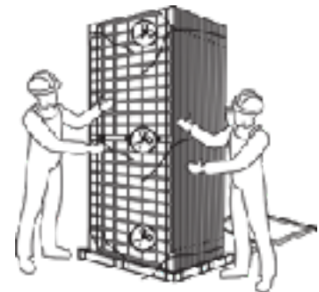
6. Cut off all the horizontal packing belts.
