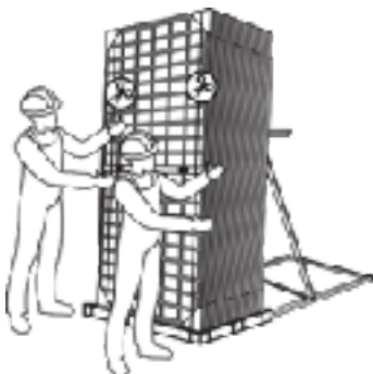
7. When there are 1-2 vertical packing belts remaining, push the module gently to tilt toward the stand supporter.
