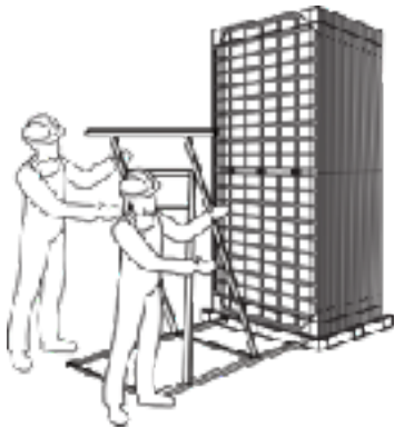
4. Place the stand supporter from the glass or back-sheetside.
