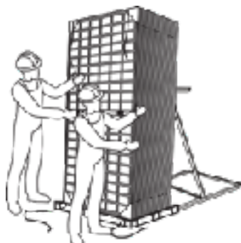
8. Cut off the remaining packing belts so that the modules rest on the stand supporter.
